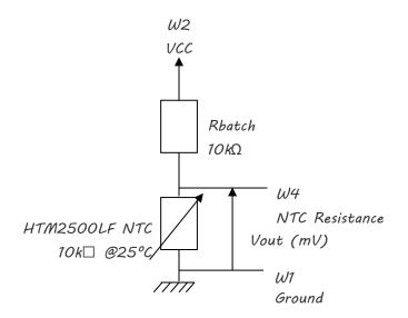
$$V_{OUT}(mV) = \frac{Vcc(mV) * NTC_{HTM \, 2500LF}(\Omega)}{R_{batch}(\Omega) + NTC_{HTM \, 2500LF}(\Omega)}$$
