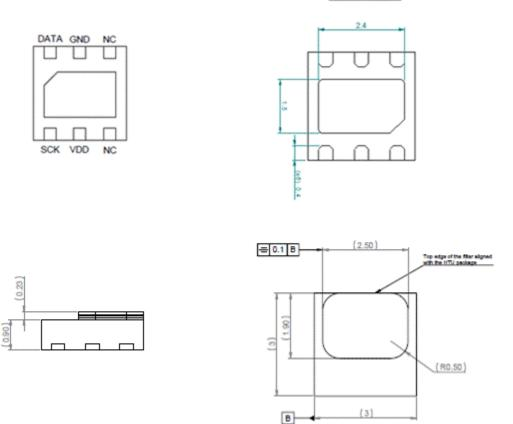
Dimensions are given in mm, tolerances are ±0.1mm. The die pad (thermal center pad) is internally connected to GND.
