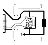
Example of HTU21P(F) sensor mounting with slits mills to minimize heat transfer
