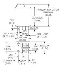
Mounting code 5 Printed circuit terminals
