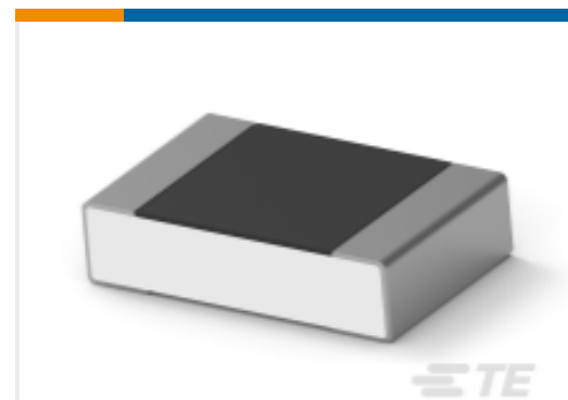
TE Part #8-2176378-9 RQ 0805 82R5 0.1% 10PPM 5K RL
