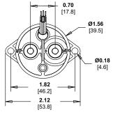
MOUNTING - 2 PLCS (HARDWARE NOT SUPPLIED) 2 X M4 BOLT, LOCKWASHER AND WASHER TORQUE: 20 IN-LBS (2.3 NM) MAX
