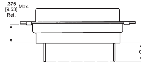
Post Extension When Used in a Standard Connector
