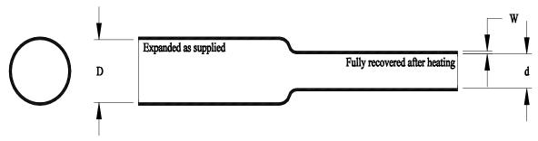
This specification covers the requirements for one type of single wall, electrical insulating, extruded tubing whose diameter will reduce to a predetermined size upon application of heat in excess of 140℃ (284℃).
