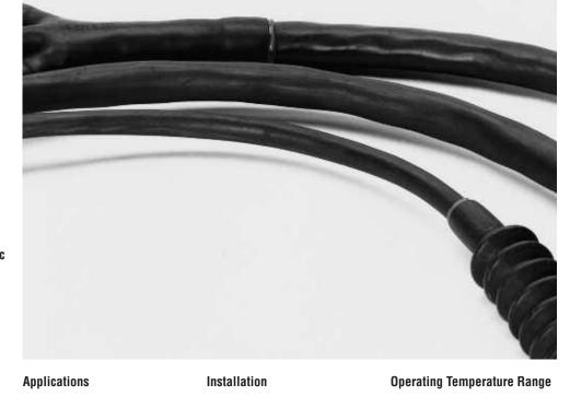
Widely used for insulation, strain relief, and abrasion protection on cable harnesses and wire bundles in the military and aerospace industries. Especially suitable for applications requiring exposure to fluids and solvents at elevated temperatures. Minimum shrink temperature: 90°C [194°F] Minimum full recovery temperature: 135°C [275°F]
