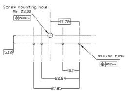
**Note :** Extra nut and washer will be provided on the screw, which will goes under PCB to fix the relay. Hex Nut S= 6.35 (width across flats), Thickness = 2.40; Washer = OD :  $\Phi$ 485±0.25, ID :  $\Phi$ 2.75±0.15, Thickness : 0.55
