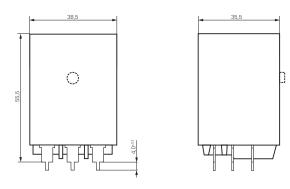
Cover with DIN-snap-on attachement (6.3mm quick connect only) horizontal vertical
