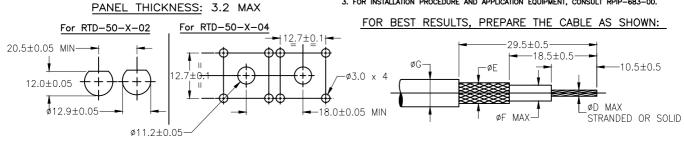
DIMENSIONS: 09MAR2020 MATERIAL FINISH DWN T.CORREIA mm CHK 09MAR2020 R.MACNAUGHT ŌŇ TOLERANCES UNLESS OTHERWISE SPECIFIED: TE Connectivity APVD 09MAR2020 N.PRZYBYLSKA PRODUCT SPEC 0 PLC  $\pm$ NAME ONE STEP CONNECTOR 1 PLC ± -2 PLC 3 PLC ± -50 OHM TNC  $\pm$ APPLICATION SPEC 4 PLC ± -SIZE CAGE CODE DRAWING NO RESTRICTED TO ANGLES 06090 C-RTD-50-Y-XX WEIGHT SCALE SHEET REV CUSTOMER DRAWING DNS 1 OF
