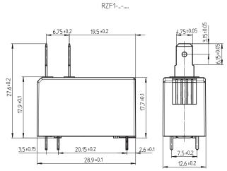
Terminal dimensions: Coil-Terminal: 0.5±0.025 Contact-Terminal: 0.5±0.01 x 0.8±0.05
