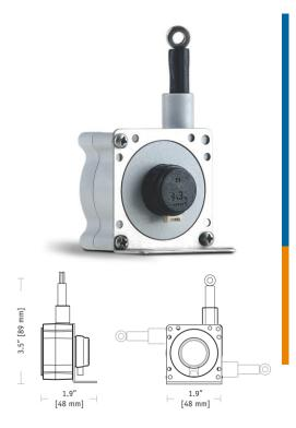
The Celesco SE1 is the digital encoder version of our compact String Pot series. The SE1 is an economical and durable device that utilizes a flexible cable, a spring-loaded spool and an incremental optical encoder to detect and measure linear position.
