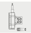
4-pin M12 connector 13 ft (4 m) 22 AWG (.34mm<sup>2</sup>) Part No. **SGD-80-3**
