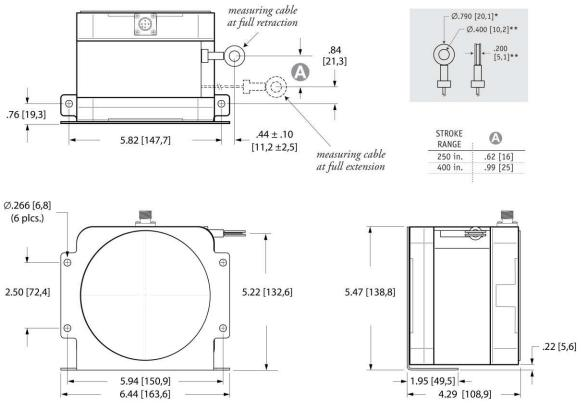
DIMENSIONS ARE IN INCHES [MM] tolerances are 0.04 IN. [1,0 MM] unless otherwise noted. \* tolerance = +.005 -.001 [+0,1 -0,0] \*\* tolerance = +.005 -.005 [+0,1 -0,1]
