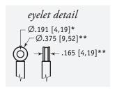
\*tolerance = +.005 -.001 [+.13 -.03] \*\*tolerance = +.005 -.005 [+.13 -.13]
