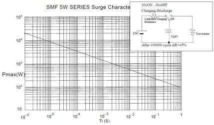
Maximum permissible peak pulse power(Pmax) as a fuction of pulse duration(Ti)
