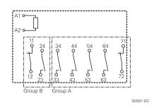
**Product code structure** Typical product code SRL 7 52 3 D 024 Type SRL Relay with force guided contacts SRL Version 7 pole **Contact arrangement 52** 5 form A + 2 form B contacts (5 NO + 2 NC) **Contact material** 3 Ag SnO Coil system **D** DC coil Coil Coil code: please refer to coil versions table (e.g. 012=12VDC)
