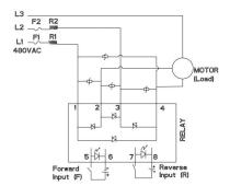
R1,R2: PROTECTION RESISTORS F1,F2: SEMICONDUCTOR FUSES
