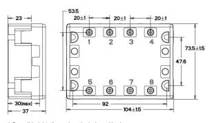
\* Overall height dimensions includes with clear cover Dimensions in mm
