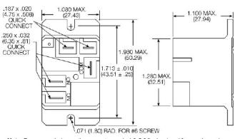
Note: Recommended mounting screw torque is 4.0-5.0 lbs.in when #6 screw is used
