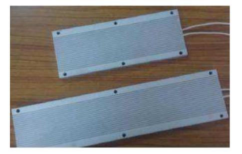
The TJT series is a range of high quality, high stability Aluminium housed low profile Power resistors designed for direct heat sink attachment. A wide range of resistance values is available in 150W to 500W when fitted to a standard heatsink
