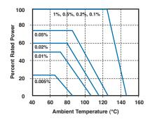
UPW Series resistors must be derated for tolerances below 0.1%. Use the graph to select tolerance versus operating temperature to determine the percentage rated power for operation. No derating is required for operation below 20 °C.
