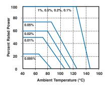
UPW Series resistors must be derated for tolerances below 0.1%. Use the graph to select tolerance versus operating temperature to determine the percentage rated power for operation.
