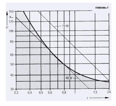
d = switching currentU = switching voltage
