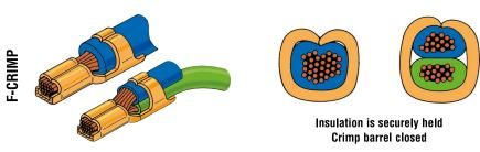
For double wire applications with different size wires always place wire with smallest outer diameter in the bottom
