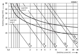
Load limit curve 1: arc extinguishes during transit time (CO contact).
