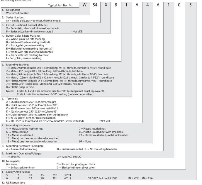
Leave Blank = UL1077 recognized breaker
