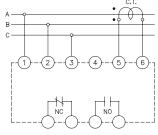
For operation on three phase, three wire
