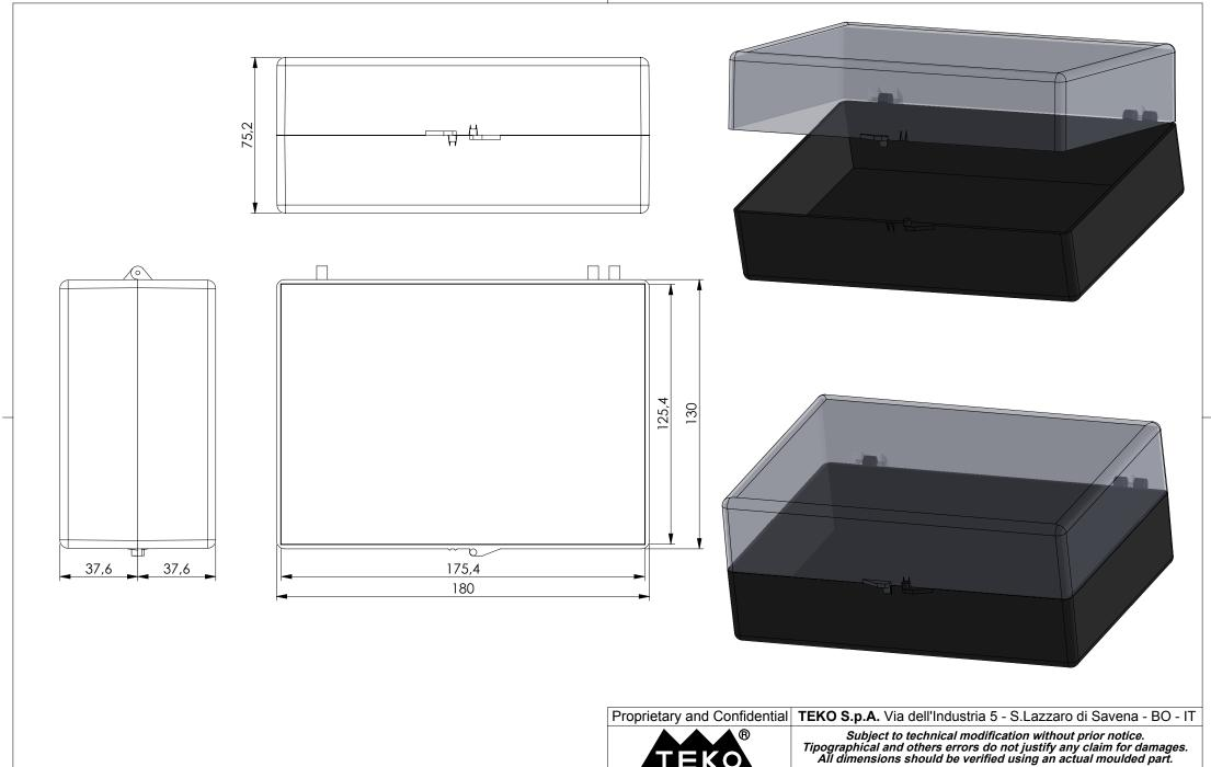
All dimensions should be verified using an actual moulded part.
