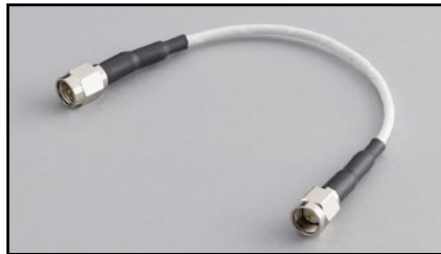
CA-405B: 15cm (6 in) RG188 coax cable terminated with an SMA male plug on each end, 50Ω impedance.
