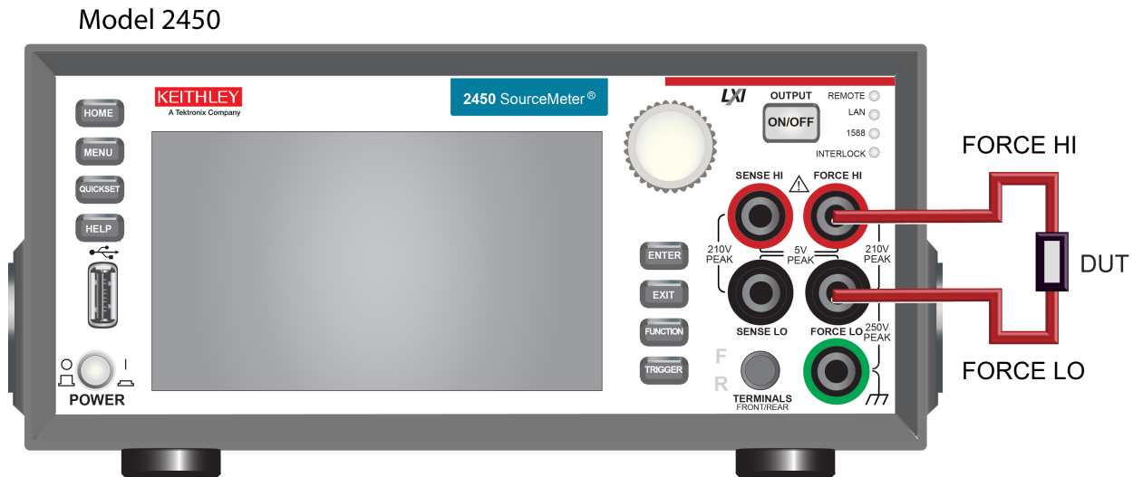
Figure 59: Model 2450 2-wire rear-panel connections
