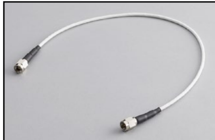
CA-406B: 33cm (13 in) RG188 coax cable terminated with an SMA male plug on each end, 50Ω impedance.
