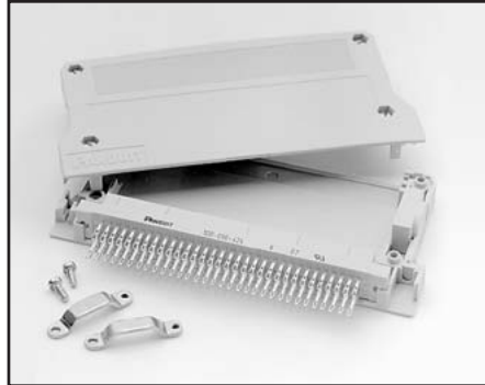
Model 7011-KIT-R: 96-pin female DIN connector with solder eyelets and strain relief. This kit can be used for assembly of custom cables to connect with the connectors on the 7011-C, 7012-C, 7013-C, 7015-C, and 7018-C switch cards. Also connects with the 7011-MTR bulkhead mount male connector. For use with: 7011-C, 7012-C, 7013-C, 7015-C, 7018-C
