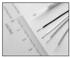
**Model 8681 Low Cost RTD:** This inexpensive RTD has small size (0.09 in  $\times$  0.09 in) and fast thermal response time.  $100\Omega$ ,  $0.385\%^{\circ}$ C element. Meets or exceeds DIN 43760-1980-A, IEC 751:1983-A, BS1904: 1984-A, and JIS C1604-1981-0.2. Can be used with Model 8680 RTD Input Probe Adapter. Measures from  $-200^{\circ}$  to  $+600^{\circ}$ C.
