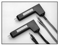
Model 5807-7 Helical Spring Point Test Leads: Two excellent Kelvin test probes for Keithley instruments that measure 4-terminal resistance. The probes have pointed tips that rotate when pressure is exerted on the handle. Good contact is assured, and the handle can be held at any angle to the measurement surface. The lead wires terminate in banana plugs. Lead wire length: 2m (7 ft).
