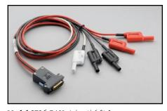
Model 3706-BAN: 1.4m (4.6 ft) banana test leads/adapter cable for Model 3706A mainframe with high performance multimeter option. Provides direct connection to high performance multimeter utilizing rear panel backplane connector. Safety banana connections to HI, LO, Sense HI, Sense LO, and AMP.
