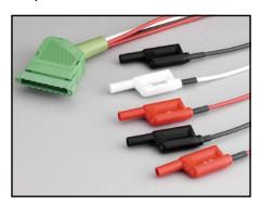
Model 2600-BAN: 1m (3.3 ft) banana test leads/adapter cable for a single Series 2600B SourceMeter channel (two needed for use with Model 2602B and 2612B). Provides safety banana connections to Hi, Sense Hi, Lo, Sense Lo, and guard.
