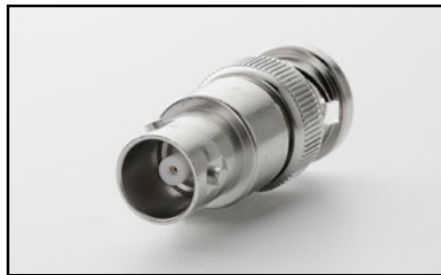
Model 237-BNC-TRX: Male BNC to 3-lug female triax adapter (guard disconnected). Terminates triax cable in BNC plug. High voltage rating for use with 7072-HV.
