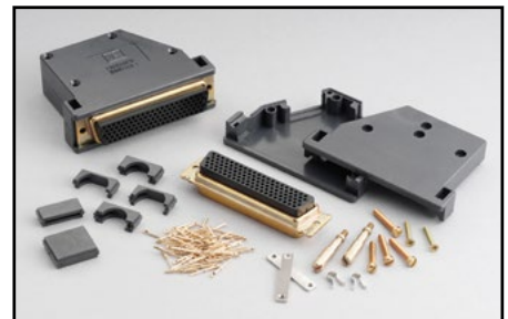
Model 3792-KIT104-R: 104-pin male D-sub connector kit that contains two male D-sub connectors with housings and 208 solder-cup contacts. Use for assembly of custom cable and harnesses compatible with Series 3700A plug-in cards.
