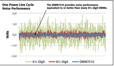
Comparison of the Model DMM7510's 1V DC noise performance with that of typical 6<sup>1</sup>/<sub>2</sub>- and 8<sup>1</sup>/<sub>2</sub>-digit multimeters. All data was taken at 1 NPLC with a low thermal short applied to the input.
