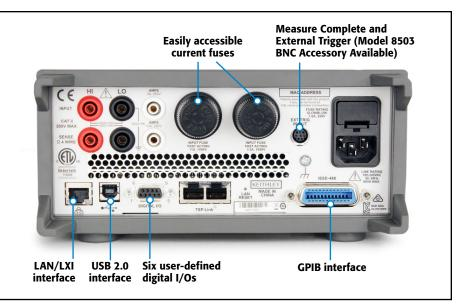
The rear panel of the DMM7510 provides connections and controls that simplify configuring multi-instrument test solutions, including input connectors, remote control interfaces (GPIB, USB 2.0, and LXI/Ethernet), a D-sub 9-pin digital I/O port (for internal/external trigger signals and handler control), and TSP-Link<sup>®</sup> jacks for connecting to other TSP-enabled instruments.
