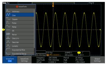
Waveform type selection in the integrated AFG.
