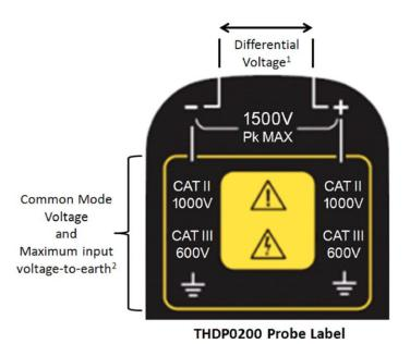
1. The differential voltageis the maximum measurable range between the (+) and (-) input leads of the probe. Beyond these limits, the output could be clipped.
