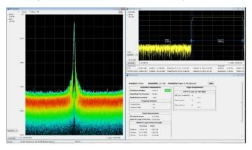
Sophisticated WLAN measurements are easy. On the 802.11g signal shown below, the spectrogram shows the initial pilot sequence followed by the main signal burst. The modulation is automatically detected as 64 QAM for the packet and displayed as a constellation. The data summary indicates an EVM of -33.24 dB RMS, and burst power is measured at 10.35 dBm. SignalVu-PC applications are available for 802.11a/b/j/g/p, 802.11n and 802.11ac to 40 MHz bandwidth.
