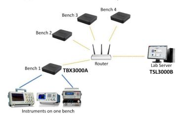
On the lab server, the TSL3000B communicates with the TBX3000A on each bench. The TSL3000B gives instructors centralized control of large fleets of instruments and gives students the ability to retrieve and save the test results online.
