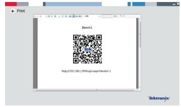
Students can login in to the web page by using their mobile device to scan the QR code, or by inputting the IP address in the web browser of their laptops. Once they have logged in, students can easily retrieve and save test results online.
