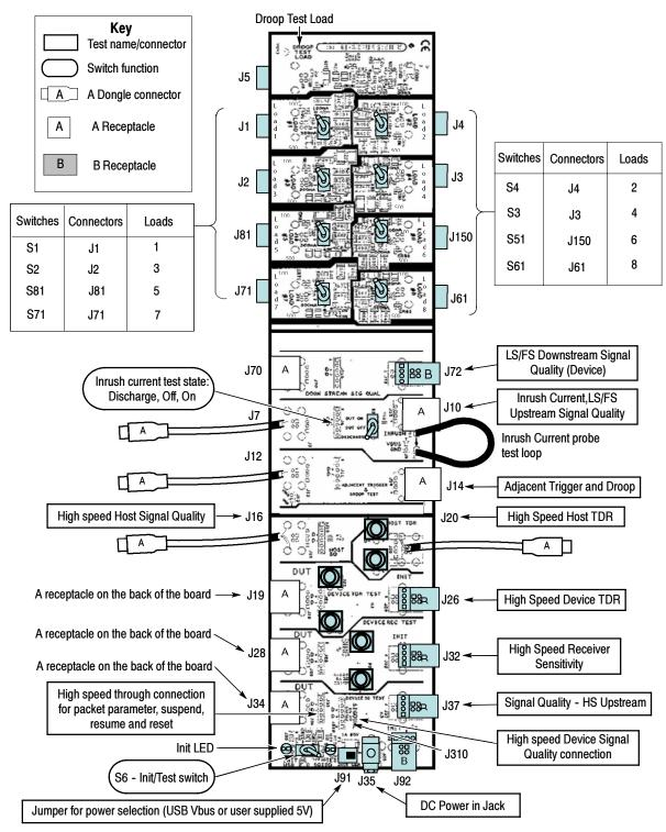
Figure 1: Fixture connections and switch functions
