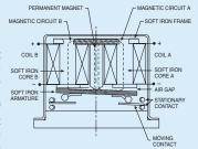
back to position B upon energizing Coil A. Since operation depends upon cancellation of a magnetic field, it is necessary to apply the correct polarity to the relay coils as indicated on the relay schematic.
