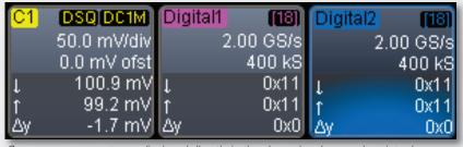
Cursor measurements are displayed directly in the channel and group descriptor boxes which are always visible on screen.
