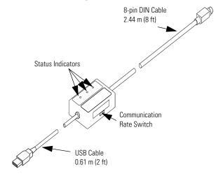
The cable operates at DH+ communication rates of 57.6 Kbps, 115.2 Kbps, and 230.4 Kbps.
