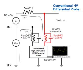
The HV differential probe measures the full common mode + sensor voltage. Therefore, the DUT load is ~100 times larger than with the HVFO. This excessive load will impact the signal fidelity and may even cause the circuit to malfunction.
