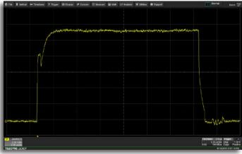
Current sinking into half-bridge phase in cascaded H-bridge – HVFO enables Miller effect to be observed clearly
