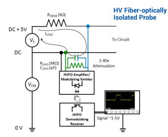
The HVFO measures only the small signal voltage with high probe input impedance; therefore, total DUT load is very small. Low tip loop inductance and 140 dB CMRR provide superior signal fidelity, noise and rejection.
