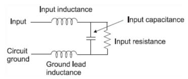
Example probe input equivalent circuit. Actual diagrams p.14.
