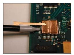
Ground Blade Used with Copper Foil
