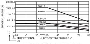
SURGE CURRENT VS. AMBIENT TEMPERATURE FIGURE 3 (SEE NOTE 3)
