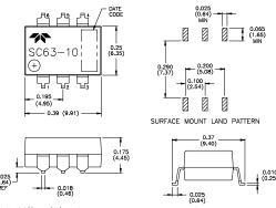
Weight: 0.035 oz. (1g) maximum Case: 6-pin dual in-line filled epoxy
