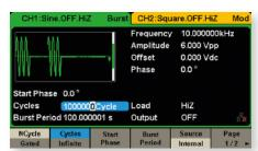
Burst mode supports 'N Cycle' and 'Gated' modes with the Burst source being configured as 'Internal', 'External' or 'Manual'.
