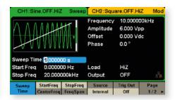
Sweep mode supports 'Linear' and 'Log' sweep, with 'Up' and 'Down' direction, and Sweep source being configured as 'Internal', 'External' or 'Manual'.
